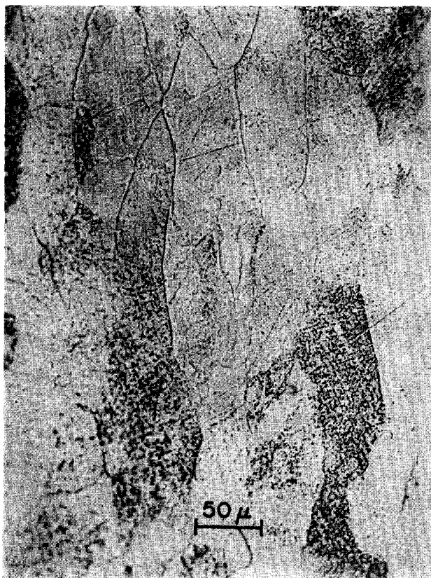
FIG. 4. Photomicrograph of 60% cold-worked platinum sample electrolytically etched in HCN solution.
