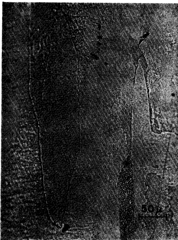
FIG. 5. Photomicrograph of 80% cold-worked platinum sample electrolytically etched in 20% HCN solution.
